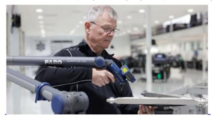
The Quantum X Series offers an up to 15% increase in accuracy compared to previous Quantum Max FaroArms.
