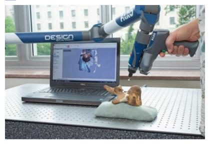
The Design ScanArm 2.5C is compatible with the FARO 8-Axis FaroArm<sup>®</sup> system, which effectively doubles the arm reach and substantively improves the ease of use, is specifically designed to address design challenges across a range of industries including Computer Graphics, Industrial Machinery, Auto Manufacturing and Engineering Services.
