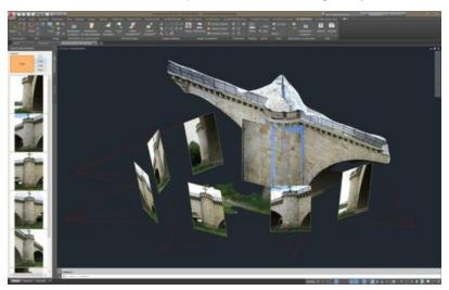
This comprehensive and innovative platform seamlessly integrates processed 3D data coming from the FARO SCENE software platform and can then support point cloud modelling (*i.e. the set of data points acquired by a 3D laser scanner that are then displayed as a visual representation of an object or area*) for the latest 2019 Autodesk design tools. The FARO As-Built platform offers three powerful options:
